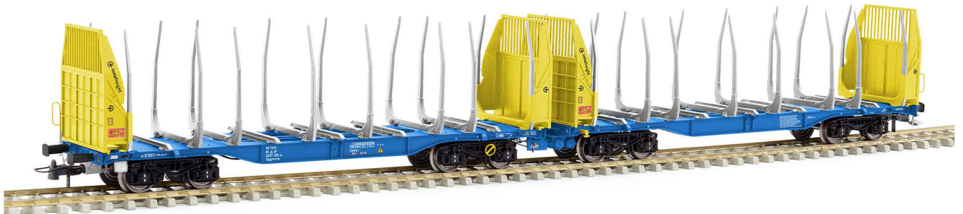
S657105 Innofreight articulated double timber transport wagon Sggmrrs | Innofreight Doppel Holztransportwagen Sggmrrs - A-IF 35 81 4657 105-6
