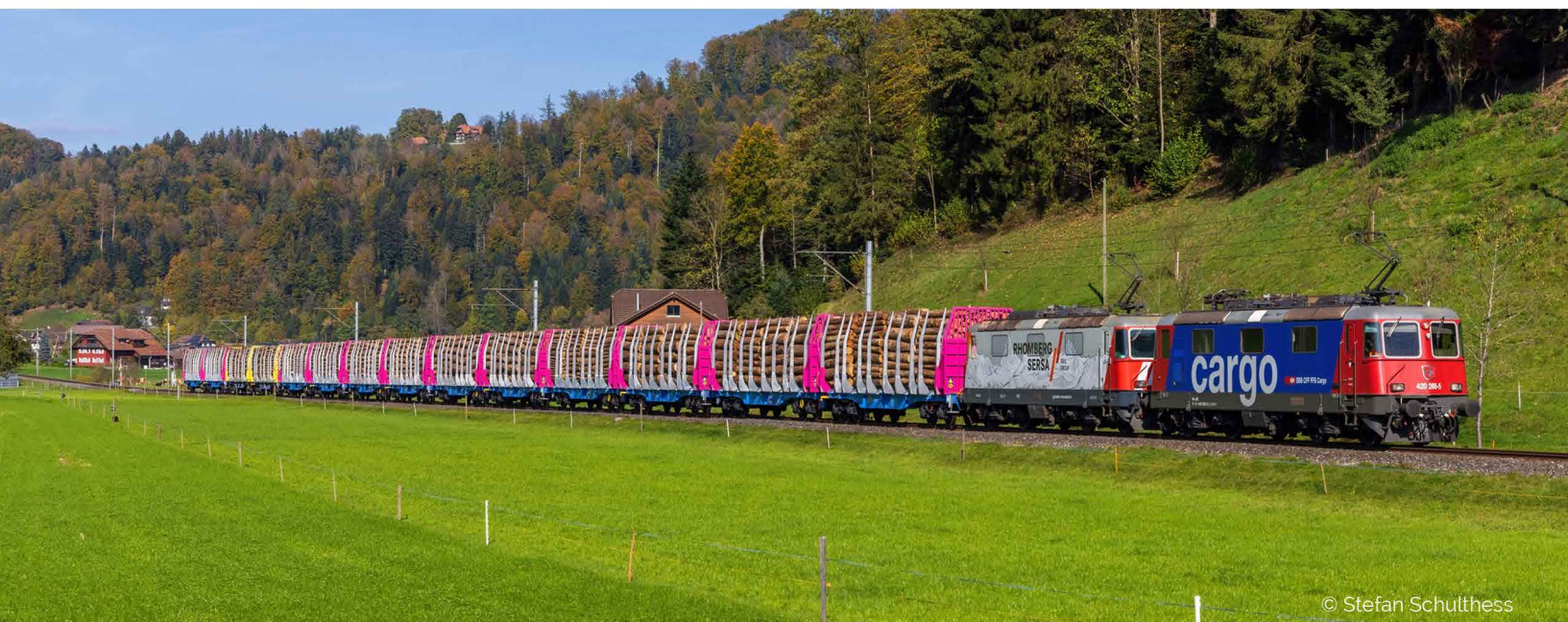
S657111 CD Cargo articulated double timber transport wagon Sgmrms | CD Cargo Doppel Holztransportwagen Sgmrms - A-IF 35 81 4657 010-8
