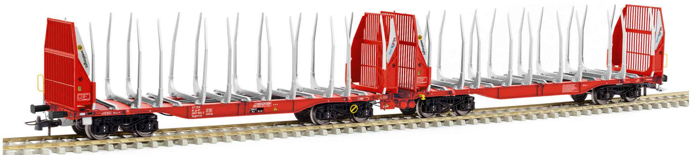
S657002 Ibercargo articulated double timber transport wagon Sggmrrs | Vagão articulado duplo transp. madeira Ibercargo Sggmrrs - A-IF 37 81 4657 002-3
