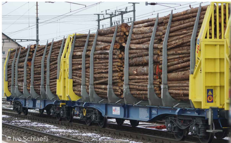
S657044 Innofreight articulated double timber transport wagon Sggmrrs | Innofreight Doppel Holztransportwagen Sggmrrs - D-IF 37 80 4657 044-6 "HLG-Berba"
