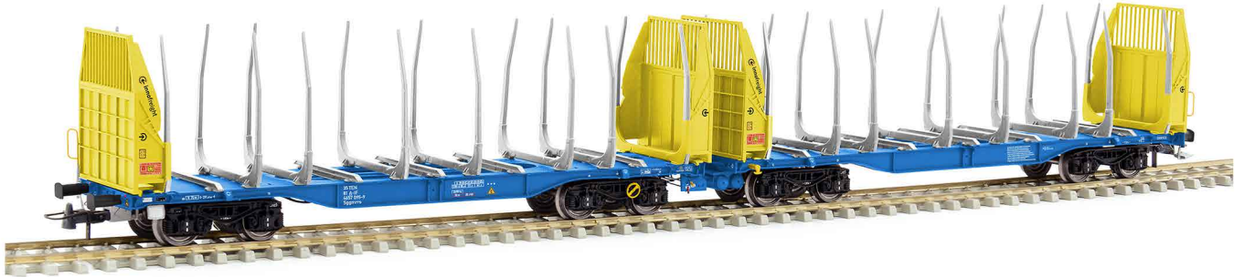
S657095 Innofreight articulated double timber transport wagon Sggmrrs | Innofreight Doppel Holztransportwagen Sggmrrs - A-IF 35 81 4657 095-9
