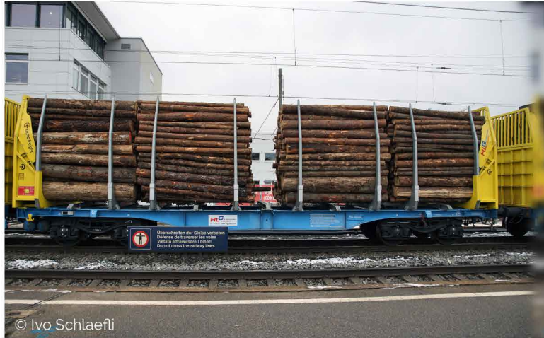
S657115 Innofreight articulated double timber transport wagon Sggmrrs | Innofreight Doppel Holztransportwagen Sggmrrs - A-IF 35 81 4657 115-5 "HLG-Berba"
