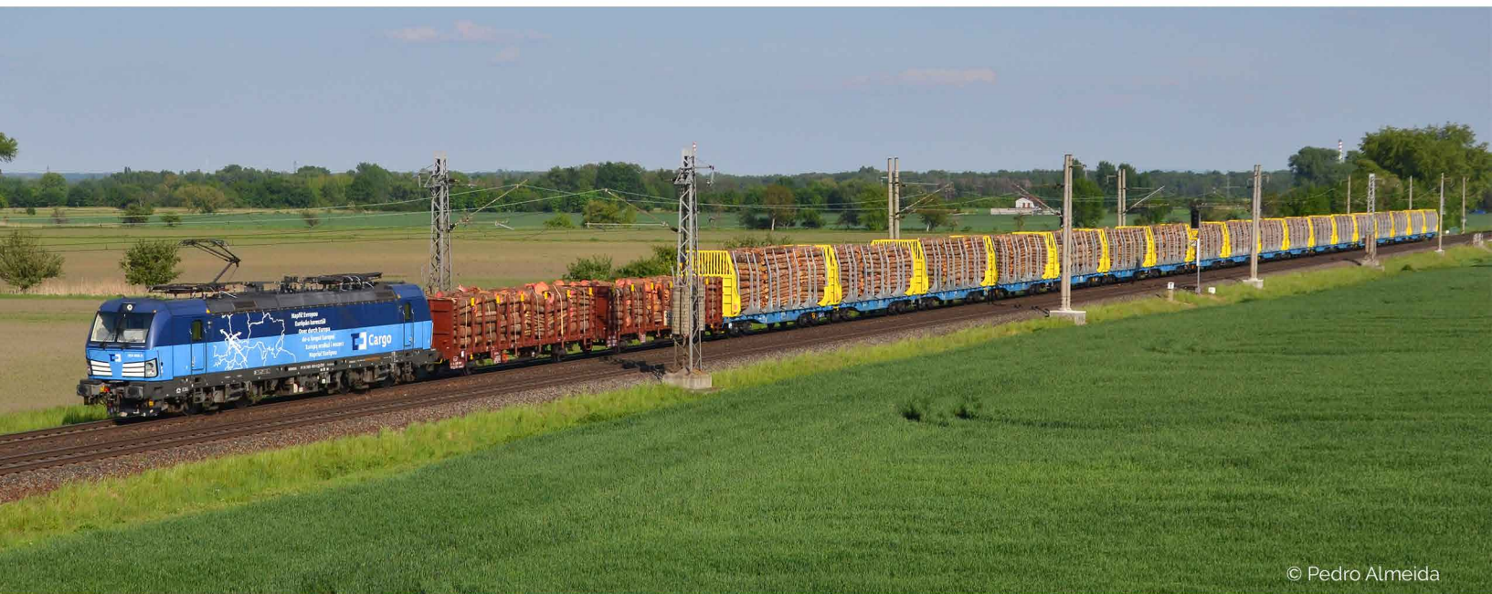
S657009 CD Cargo articulated double timber transport wagon Sgmrss | CD Cargo Doppel Holztransportwagen Sgmrss - A-IF 35 81 4657 009-0
