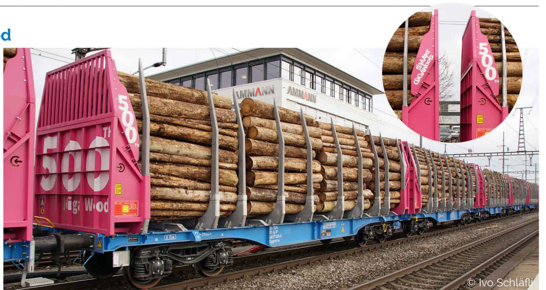
S657325 Innofreight articulated double timber transport wagon Sggmrrs | Innofreight Doppel Holztransportwagen Sggmrrs - A-IF 35 81 4657 325-0 "500TH Smart GigaWood"
